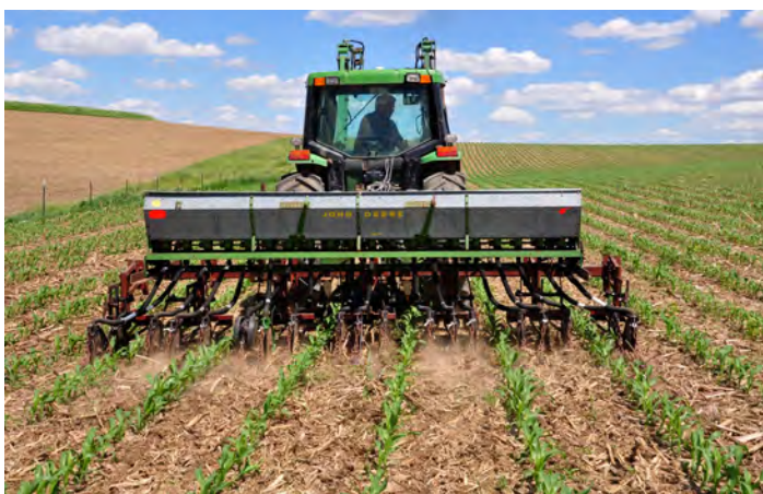
A tractor drags an old drill adapted to interseed cover crops among rows of corn seedlings on the farm of Bryce Irlbeck and his father Brian, in Carroll County, Iowa.
