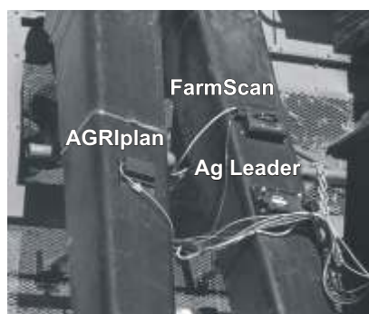
Agri-Plan, FarmScan, and Ag Leader sensors mounted on chutes 3 and 4 of the NESPAL John Deere 9965 cotton picker during evaluation. Sensors were also mounted on chutes 1 and 2.
