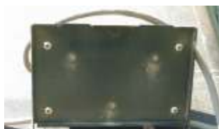
Yield monitor sensor in an open position. This sensor has 3 photo detectors.
