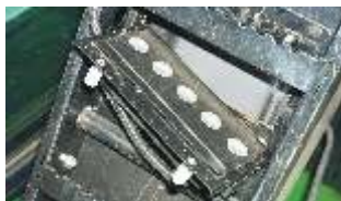
Yield monitor sensor in an open position. This sensor has 5 photo detectors.
