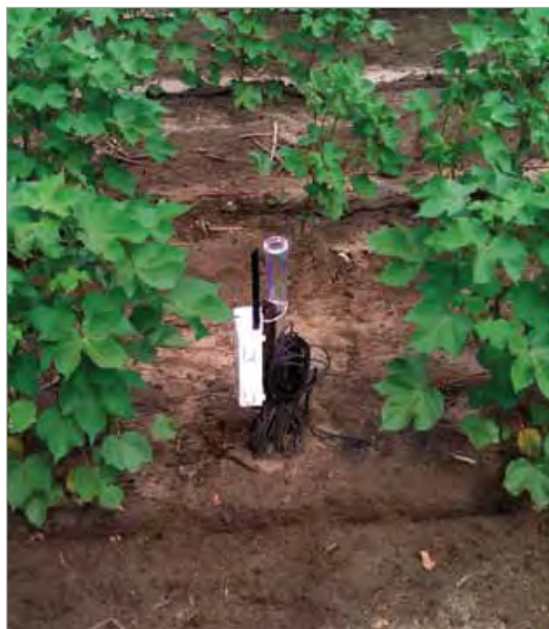
Figure 6.4 – A Decagon EM-50g data logger installed in-line with cotton plants.
