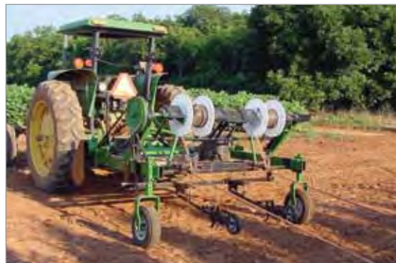
System used to install surface drip tape.
