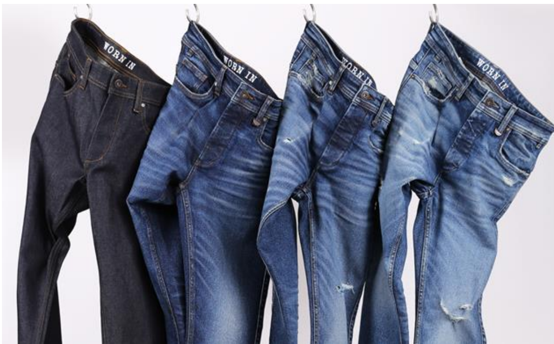
Figure 1. A series of sample garments produced by Soorty denim mills to demonstrate laser finishing techniques from unprocessed (left) to heavily altered (right).
