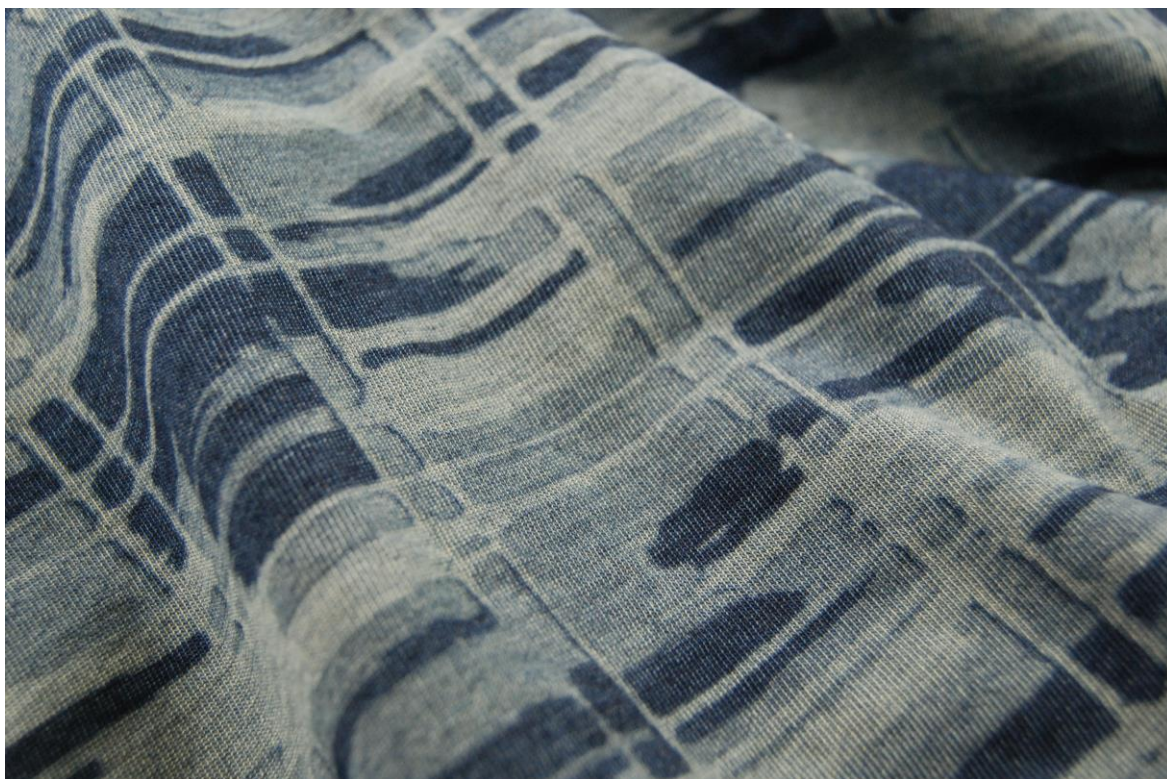
Figure 8. FABRICAST SK-2060-2A Marking an image with a laser on a medium weight indigo dyed knit
