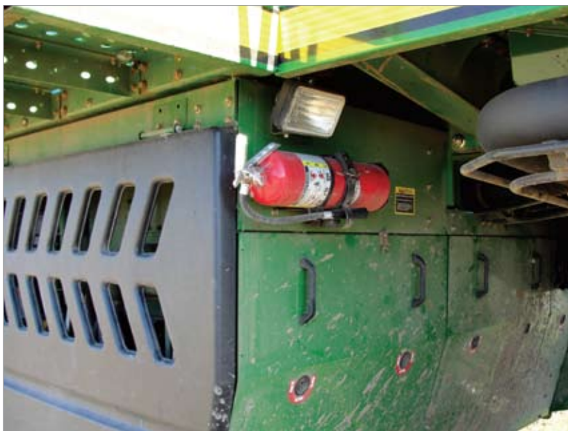
Engine compartment type ABC fire extinguisher.
