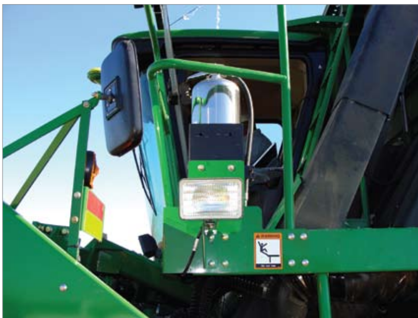
Platform water-based fire extinguisher.
