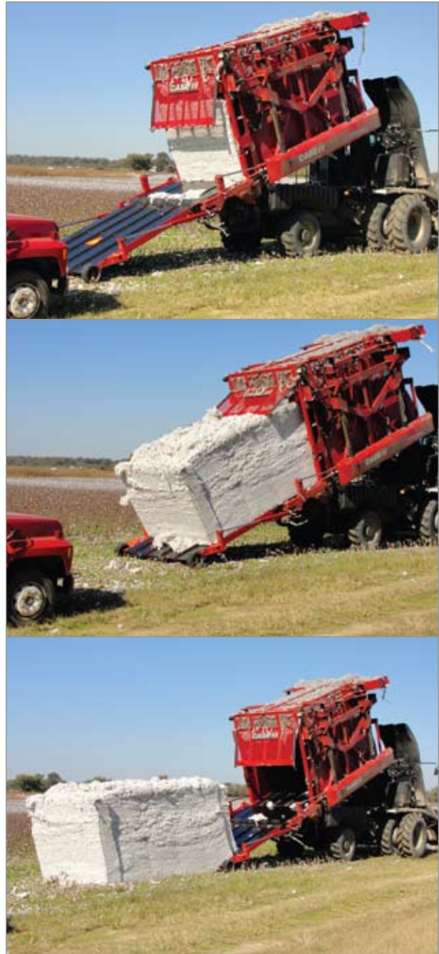
Case IH onboard module building picker unloading sequence.
