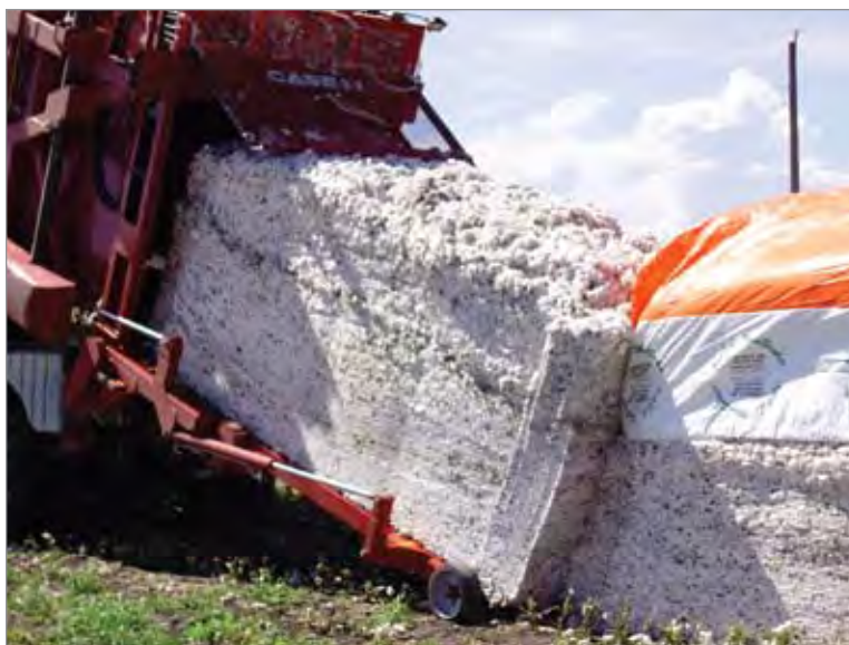
Figure 14 Half-length module unloaded too close to another module. Notice how the first module is pushed backward at the top. If this occurs before the module is covered, cotton will often fall off the back of the first module. Note also the offset between the two modules. This offset will make picking up the two modules together more difficult.
