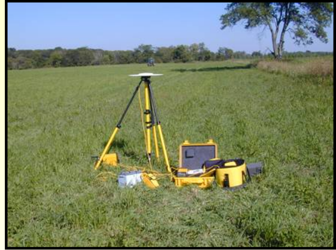
RTK Base Station with radio
