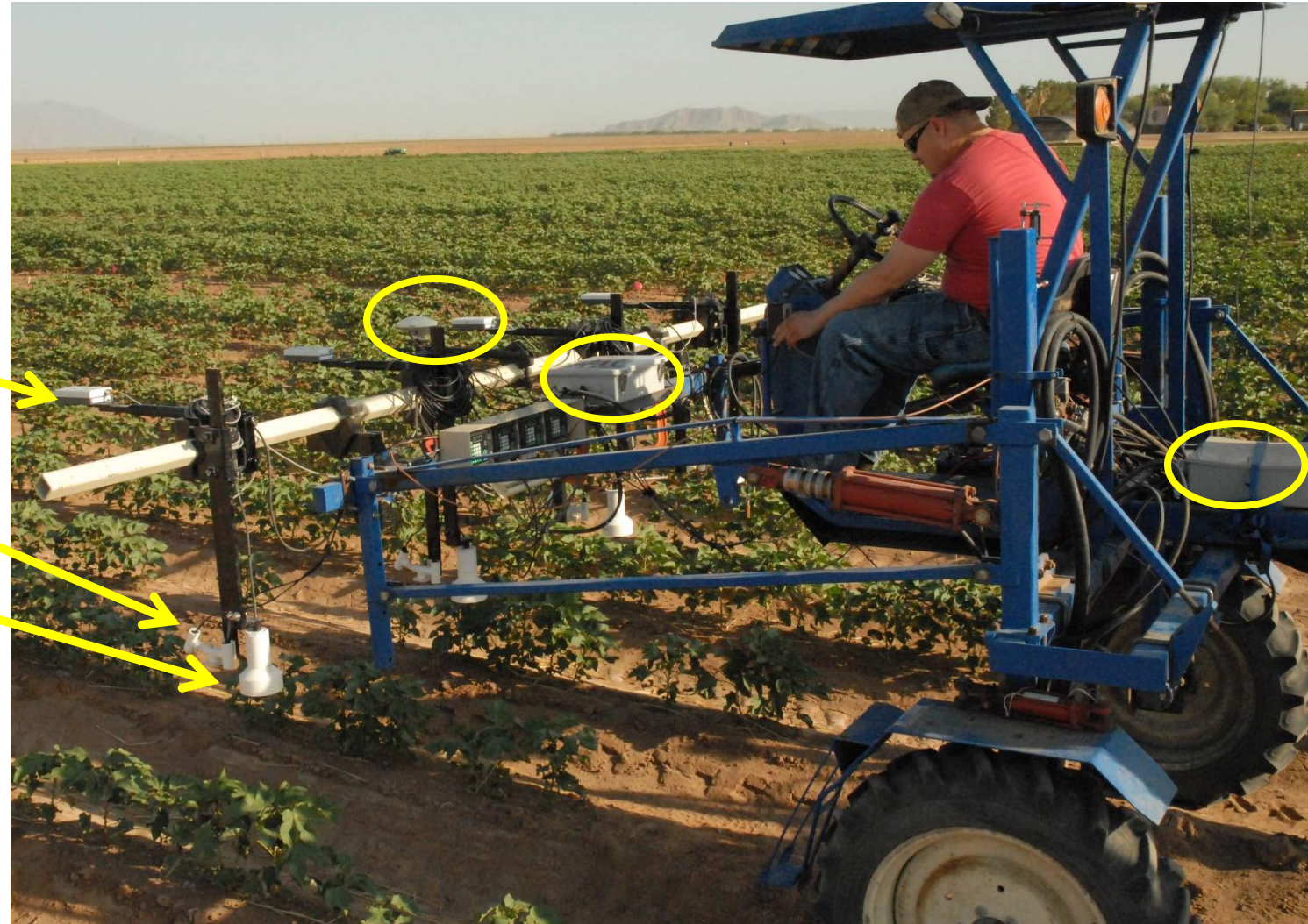
Modified high-clearance tractor
