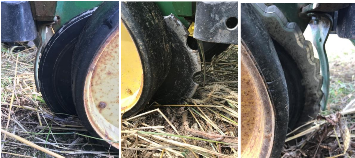
Figure 3: Smooth (a), Notched (b), and serrated (c) disk openers used.
