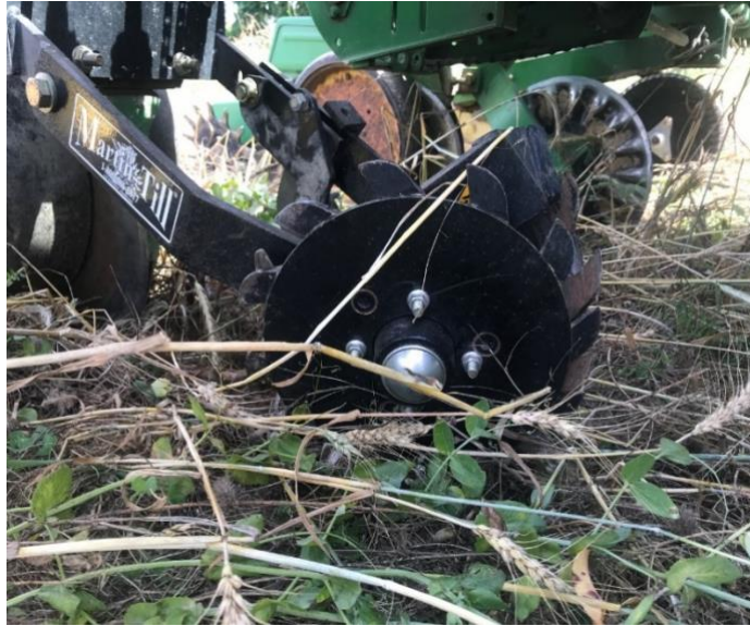
Figure 9: While the serrated double disk performed well during 2018, significant decreases in hairpin ratings were not noted from this treatment during 2019 (pictured on left). The razor wheel performed extremely well during 2018 and 2019 (pictured on right).
