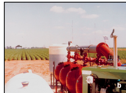
Figure 7. Laying subsurface drip (a) and the pump that maintains the flow of water through the system (b).
