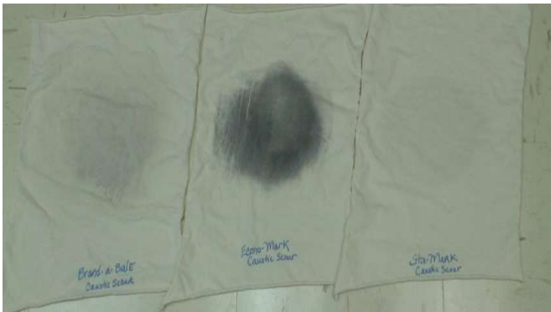
Figure 3: Sprayed fabric after caustic scour (Left to Right: BRAND-A-BALE®, ECONO-MARK, STA-MARK®)
