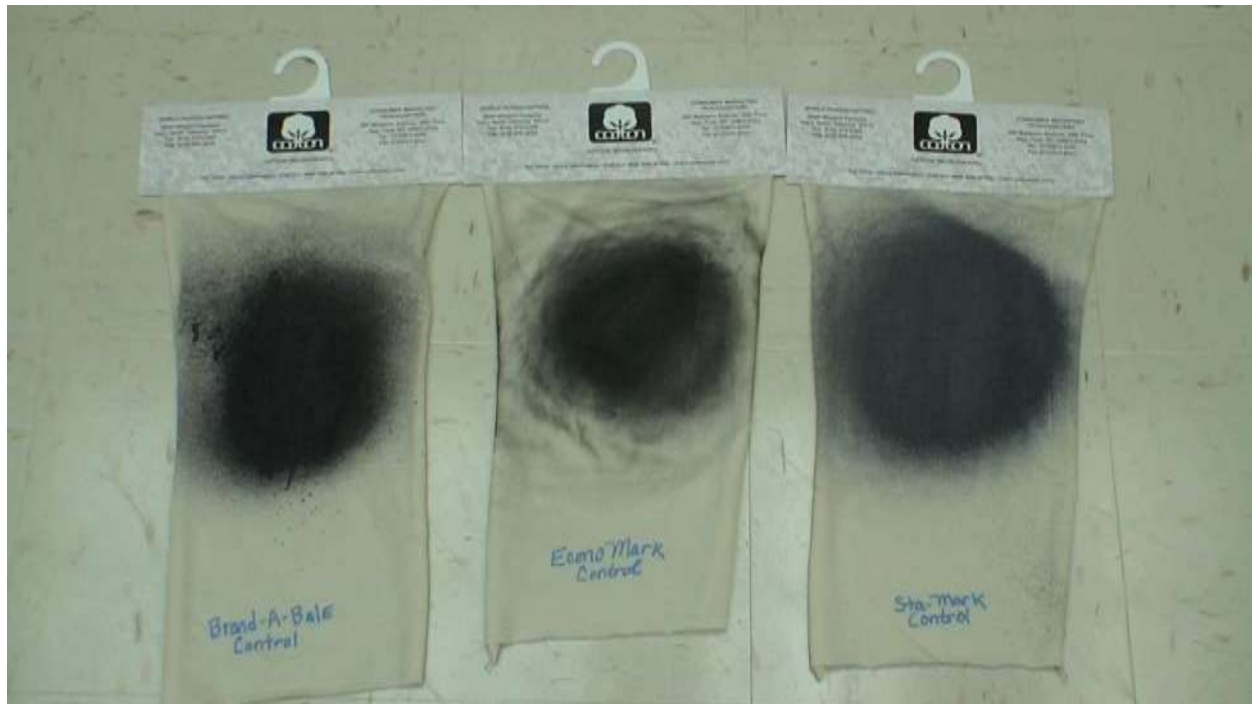
Figure 1: Sprayed fabric controls after drying (Left to Right: BRAND-A-BALE®, ECONO-MARK®, STA-MARK®)
